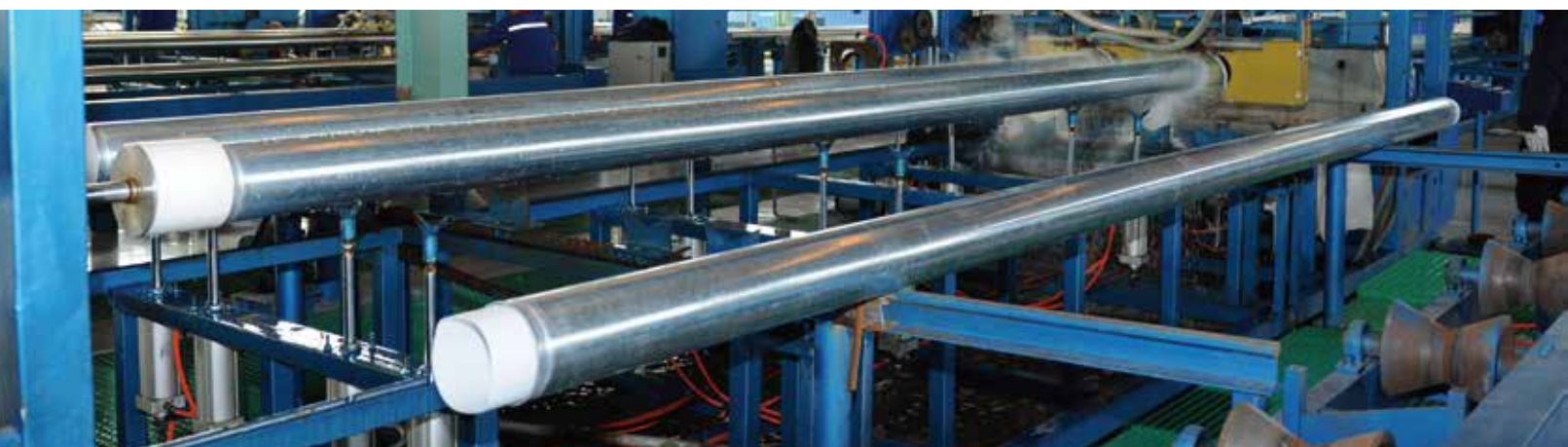
Steel Pipe of Lining Plastic Production Line
